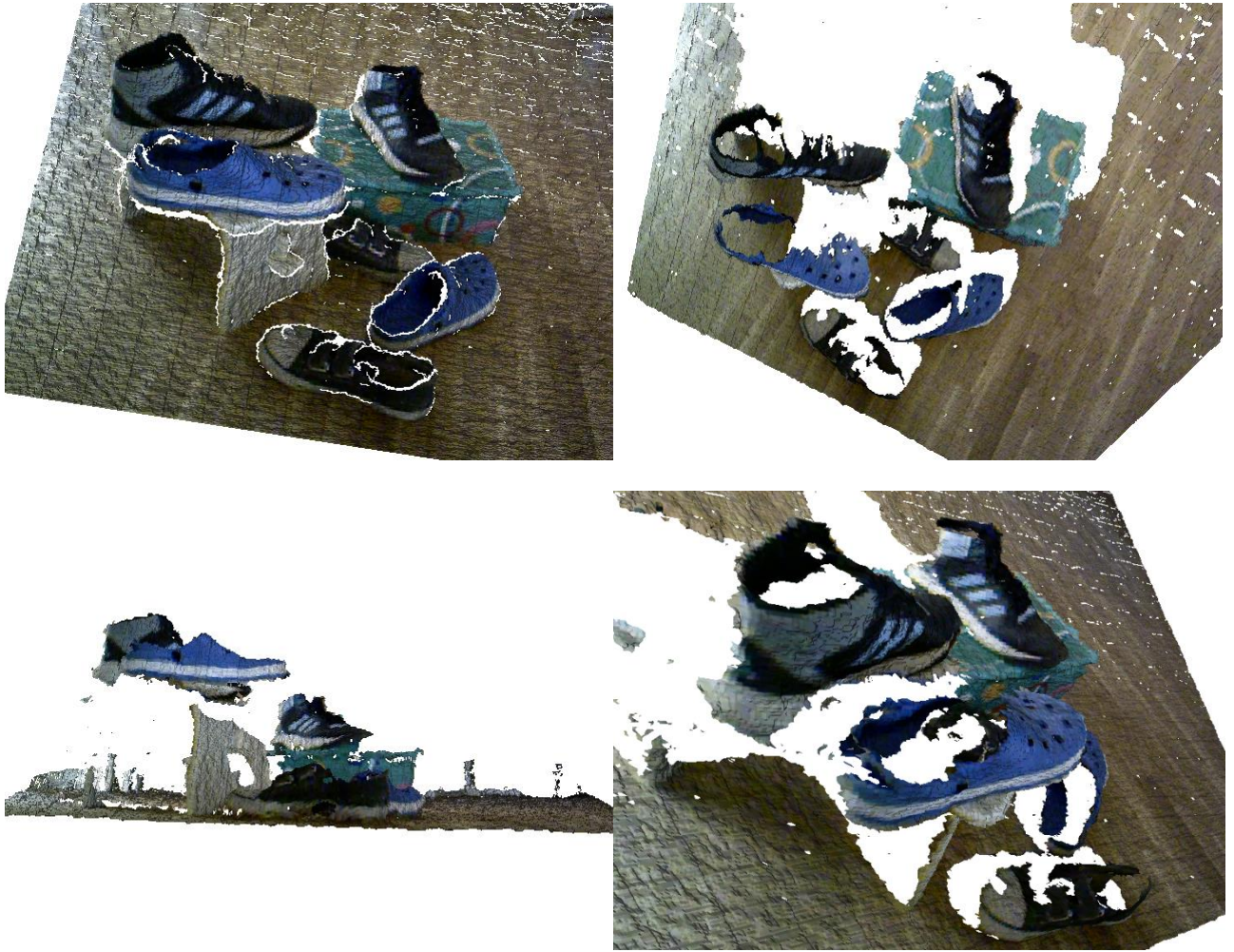
Fig. 2. Triangular mesh created from RGB and depth image shown in Fig. 1 viewed from four different viewing angles.
